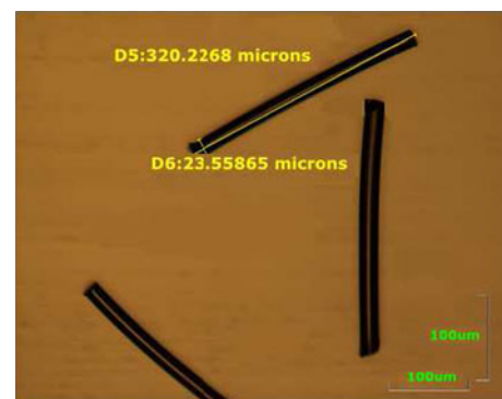
Fig. 2 Fibers microscopic image. Diameter and length of a sample fiber are given
