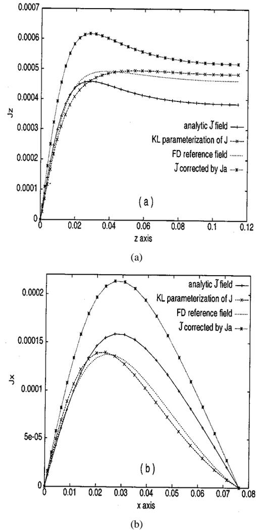
Fig. 3. Comparison of current density fields (configuration  $\mathcal{A}$ ). (a)  $J_z$  at  $x = 0.0234$  m. (b)  $J_x$  at  $z = 0.0387$  m.
