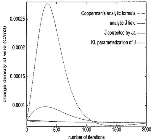
Fig. 6. Evolution of charge density at the wire (configuration  $C$ ).
