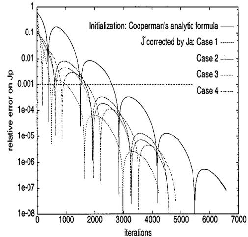
Fig. 7. Convergence histories for different values of  $x_{i_0}$  (configuration  $B$ ). Case 1:  $x_{i_0} \simeq 0.35h_x$ ; case 2:  $x_{i_0} \simeq 0.46h_x$ ; case 3:  $x_{i_0} \simeq 0.57h_x$ ; case 4:  $x_{i_0} \simeq 0.69h_x$ .
