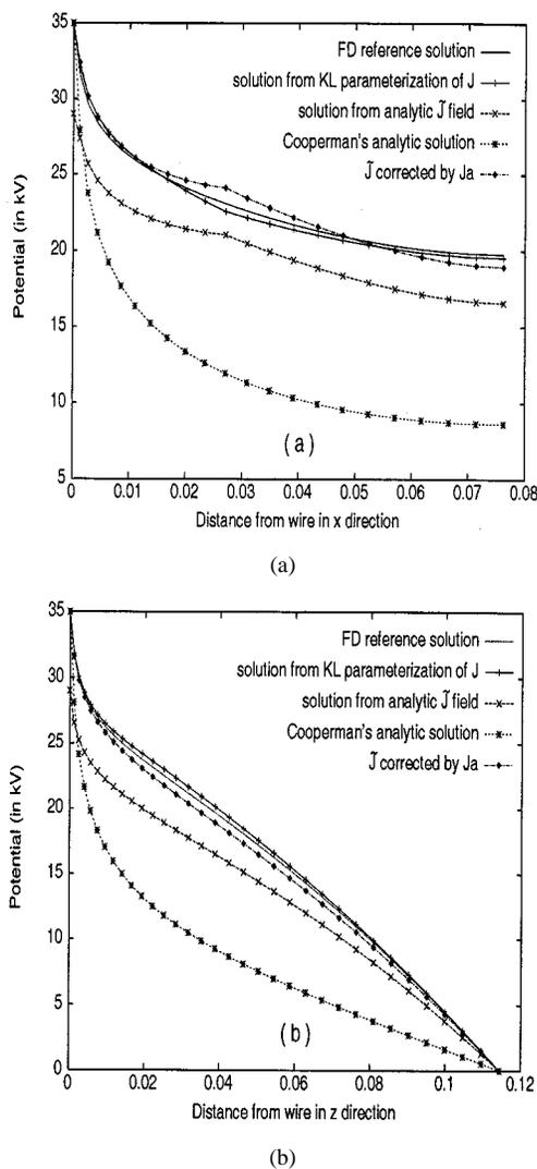
Fig. 4. Comparisons of electric potential fields (configuration  $C$ ). (a) Potential along AB. (b) Potential along AD.
