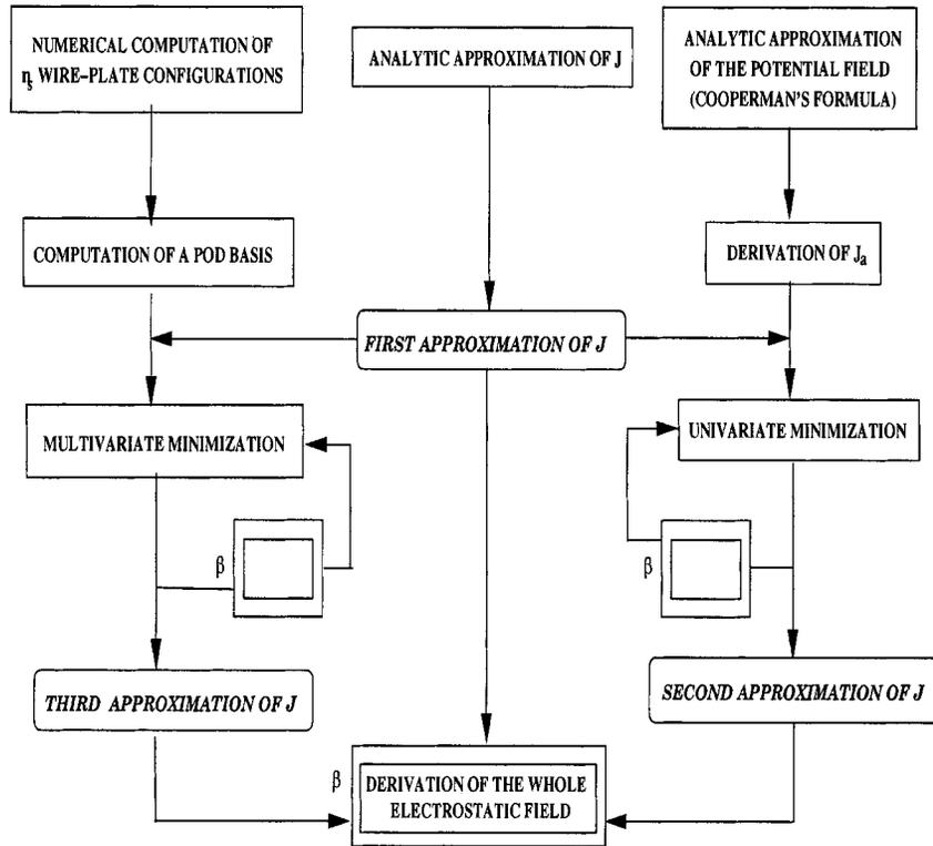
Fig. 2. Flowchart of the different proposed procedures for the initialization of the electrostatic field. The box  $\beta$  in the figure corresponds to the procedure described in Section III-A.
