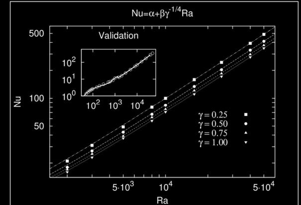
Figure 3 Nusselt number vs Rayleigh number for different values of the anisotropic parameter  $\gamma$
