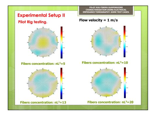
Experimental Setup II Pilot Rig testing.
