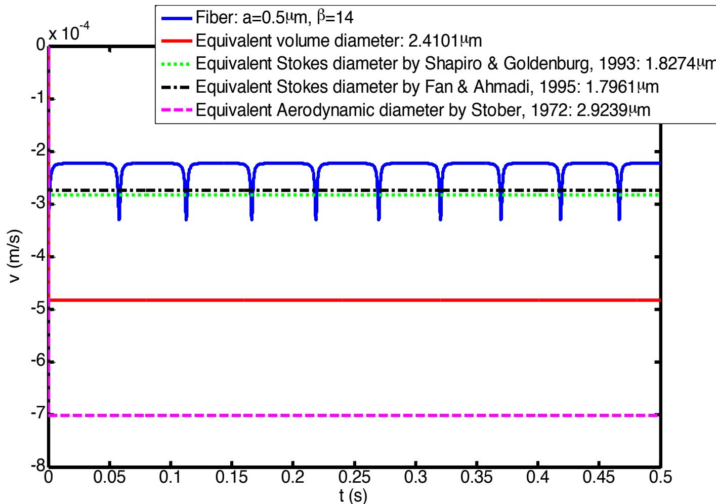
Comparison of sedimentation terminal velocities of fibers and equivalent spheres.
