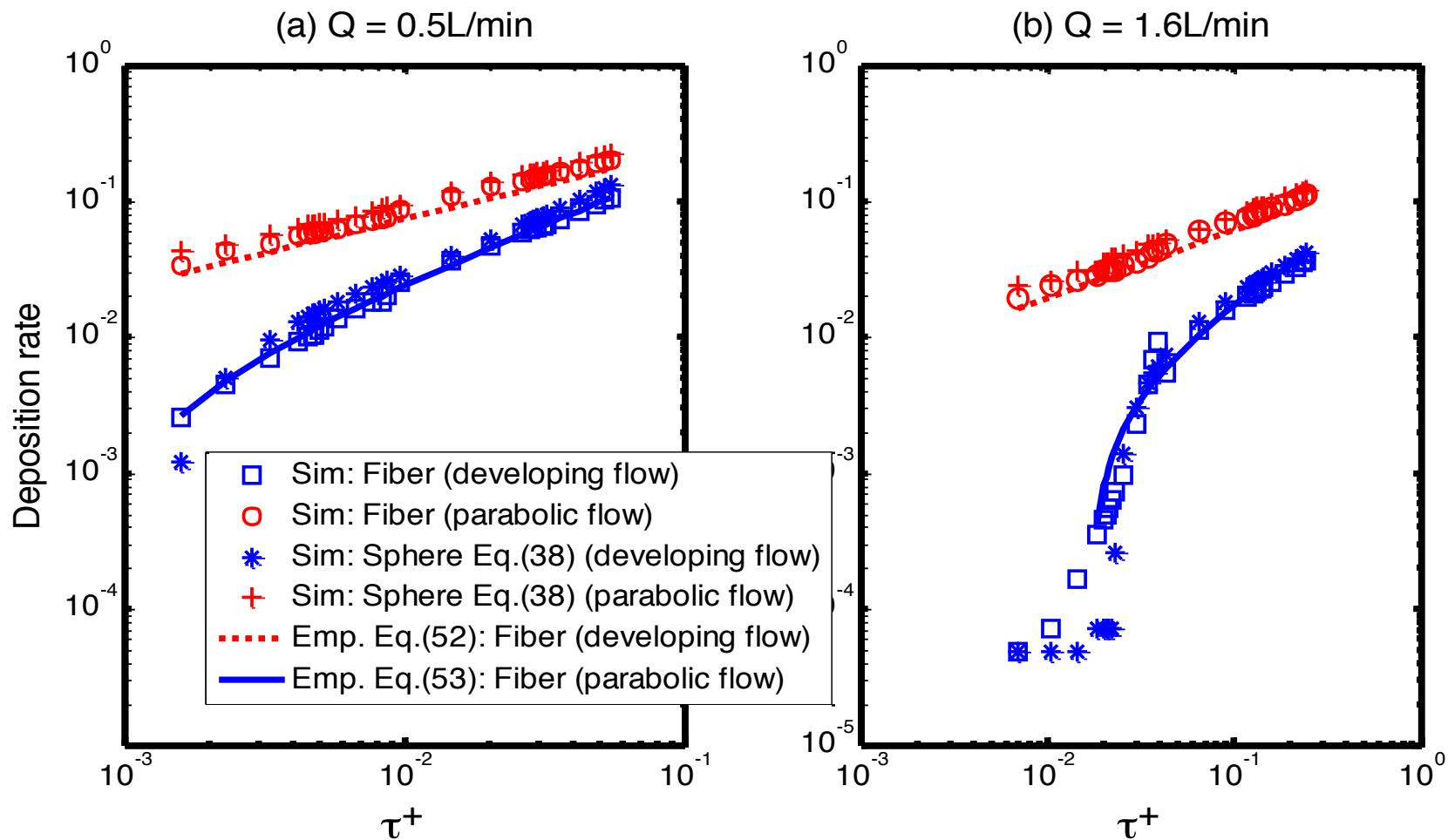
**Comparison of deposition rates of the glass fibers in the horizontal pipe in developing flow and in parabolic flow**
