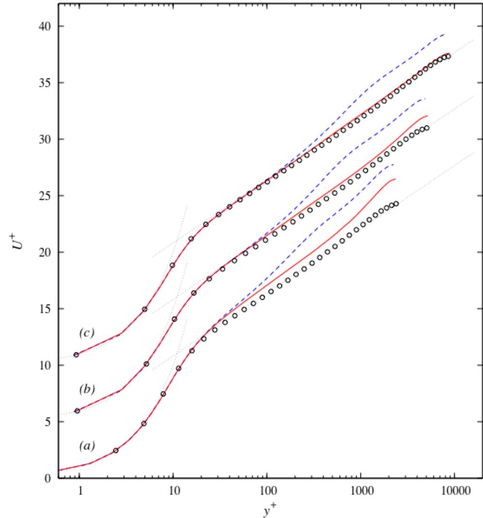
Mean velocity profiles in plane channel flow. SA-WMLES
