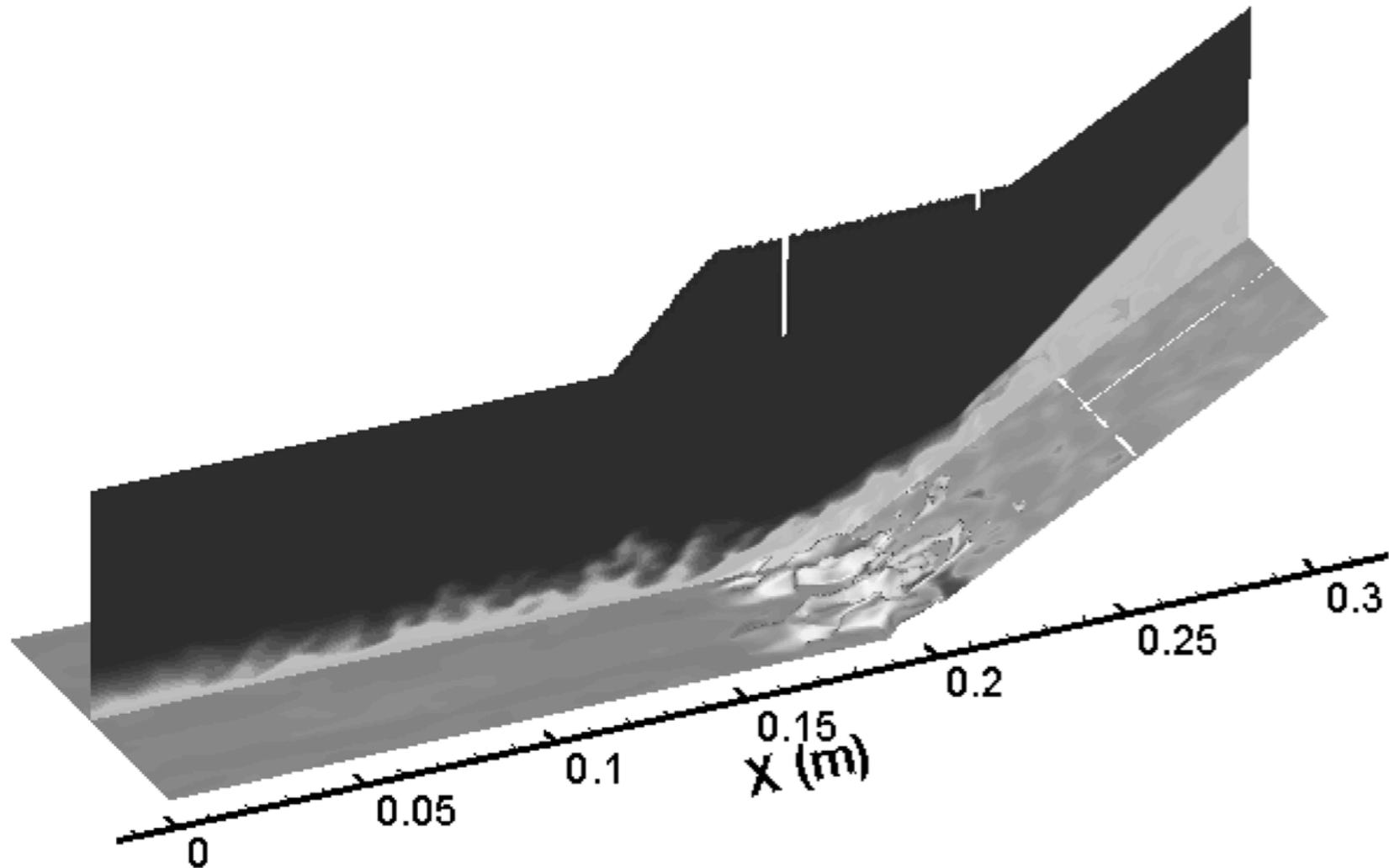
**Fig. 5** Isosurfaces of zero axial velocity shaded by temperature.
