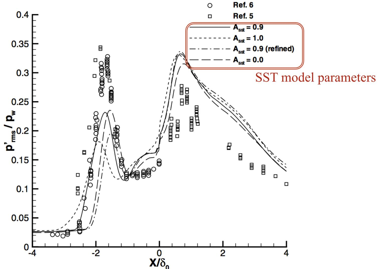
Fig. 14 The rms pressure-fluctuation distributions normalized by local wall pressure.
