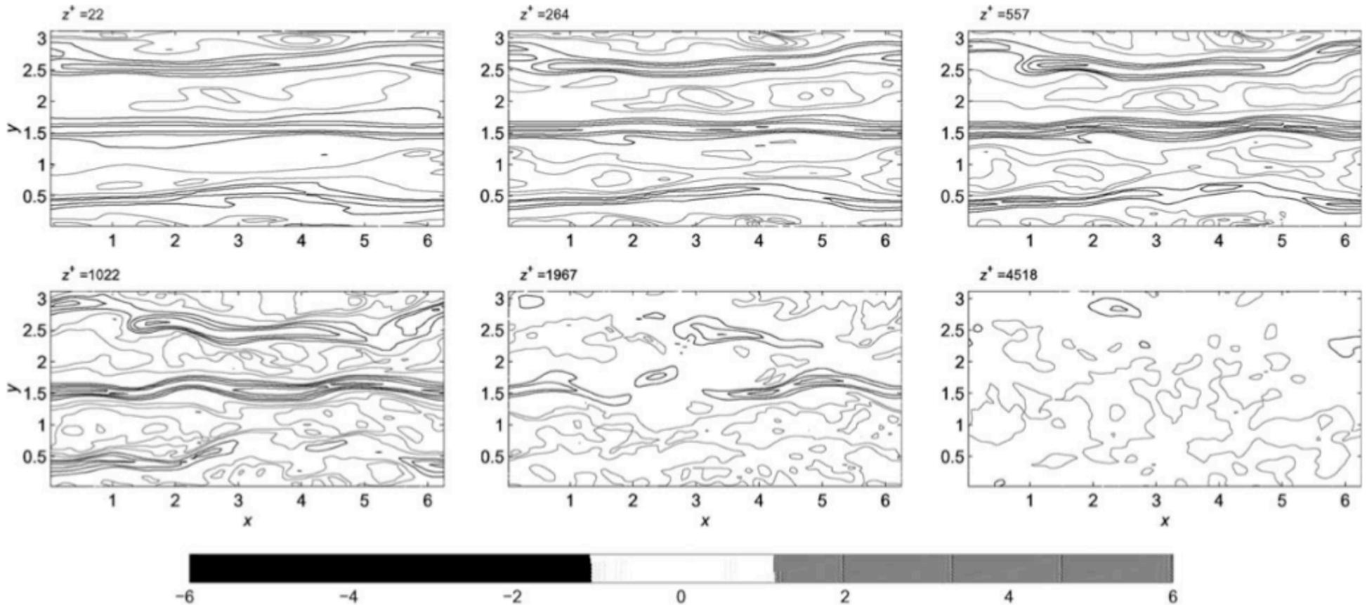
Contours of streamwise velocity fluctuations in planes parallel to the wall
