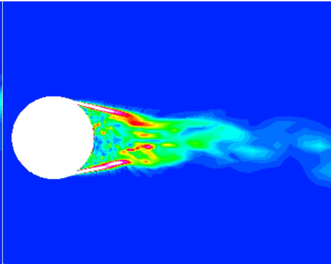
Turbulent separation,  $Re=1100k$
