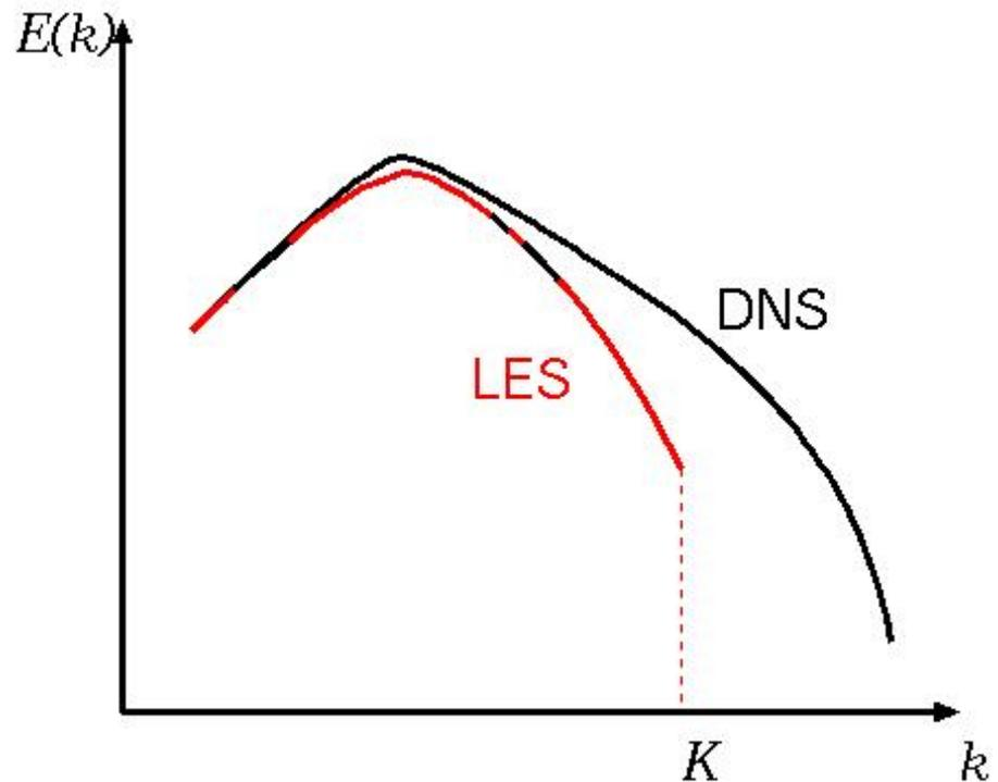
$K = \text{cutoff wavenumber} \propto 1/\Delta$  (filter width)
