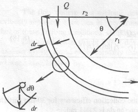
Figure 8.5 Turbulent cyclonic flow
