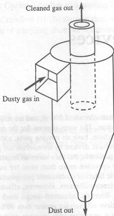
Figure 8.1 Schematic diagram of a tangential inlet reverse flow cyclone
