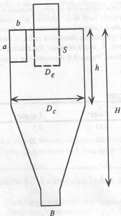
Figure 8.6 Dimensions of a standard cyclone
