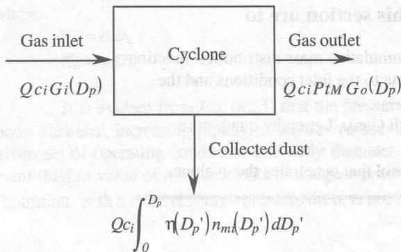
Figure 8.7 Material balance on particles finer than  $D_p$
