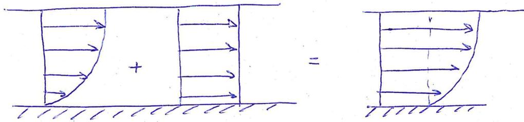
$$\Phi = \int_0^w \int_0^\delta v_x(y) dy dz = w \left[ \underbrace{\frac{1}{2\mu} \left( \frac{\partial p}{\partial x} \right) \left( \frac{y^3}{3} - \delta y^2 \right)}_{-\frac{2}{3} \delta^3} \Big|_0^\delta + U \cdot \delta \right]$$
