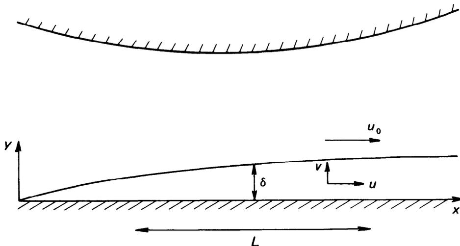
FIG. 11.1 Boundary layer on flat wall of channel: definition sketch.
