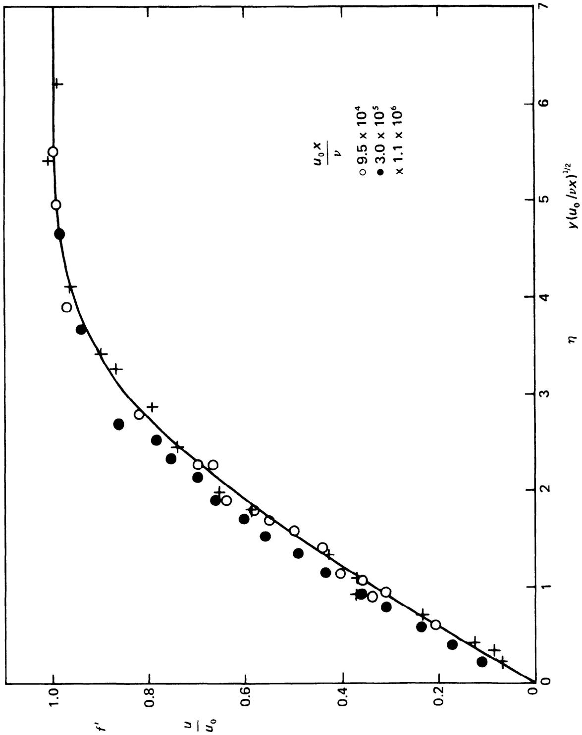
Fig. 11.2 Theoretical Blasius profile and experimental confirmation from Refs. [141] and [249].
