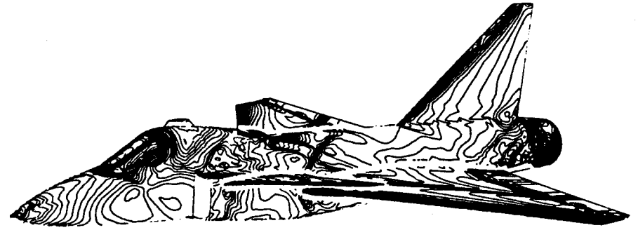
Fig. 1.4. Surface pressure distribution on a typical military aircraft. Surface pressure contours, \Delta C_p = 0.02 (after Arlinger, 1986; reprinted with permission of Japan Society of Computational Fluid Dynamics)
