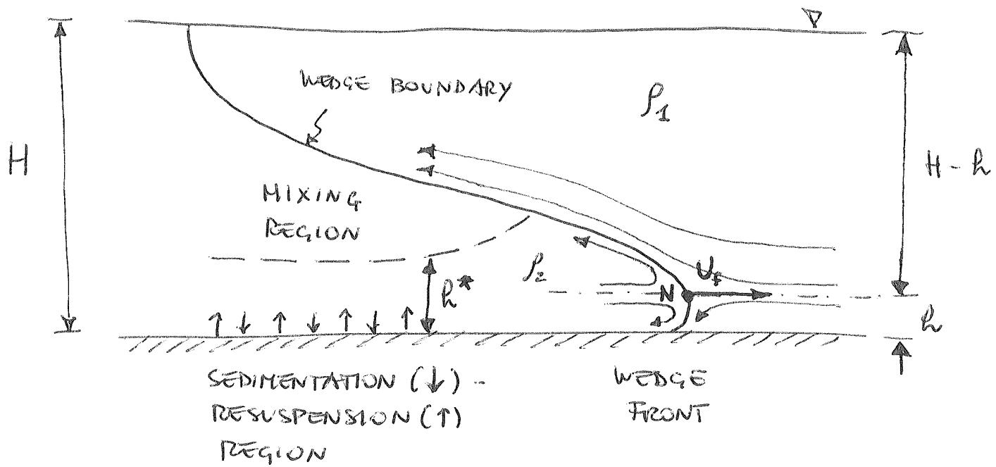
The intrusion of the heavier fluid into the lighter fluid is characterized by a frontal region culminating into the so-called "nose" (point N in the schematic), which advances with velocity  $U_f$ . Upstream of the nose, two main regions can be found :
